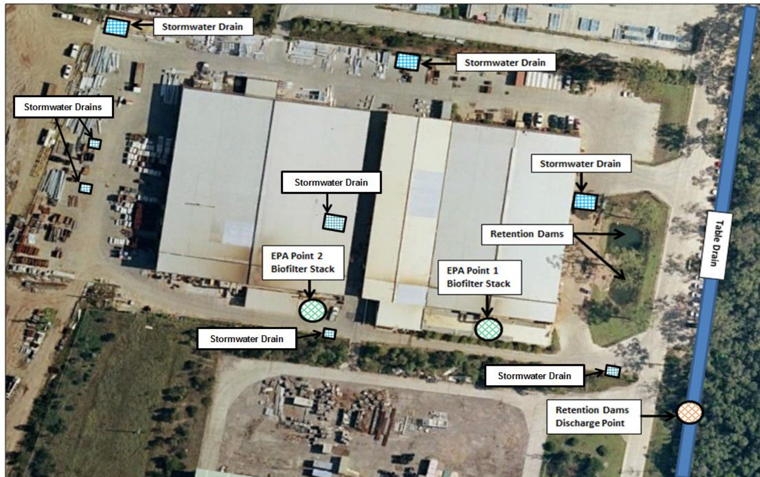
Figure 2-3: Hunter Galvanizing site map with stormwater drains, retention dams and discharge points
