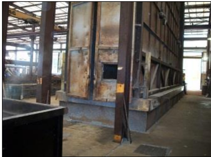
Figure 1-5: Plant 1 galvanizing bath with enclosed kettle hood
